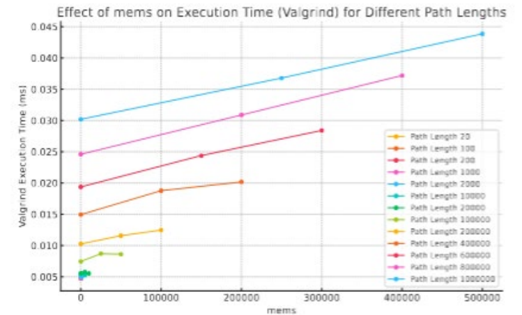
Figure 1. Graphical representation of memory access frequency and execution time correlation.
